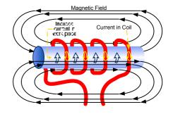
A source of high frequency electricity is used to drive a large alternating current through a coil. This coil is known as the work coil. **See the picture opposite**.
